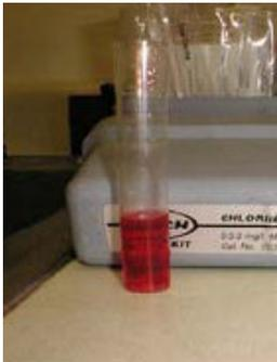
Make sure the chlorine has been removed from the water system. It is recommended that a sample be collected a couple days after the well is disinfected. **Do not use the water for drinking, cooking, or food preparation until it tests free of coliform bacteria.** Follow the procedure for collecting a water sample given on the first page of this fact sheet.
